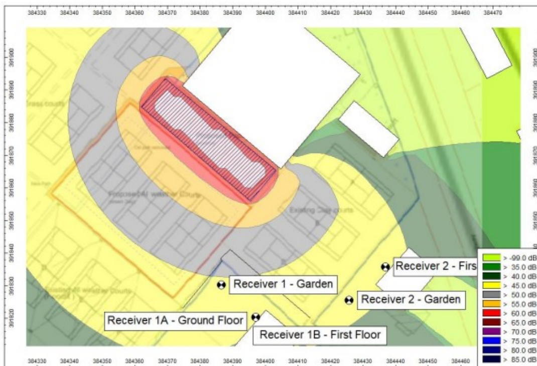
Figure 2.2: Noise contour of Padel Court propagation at 4 m height
