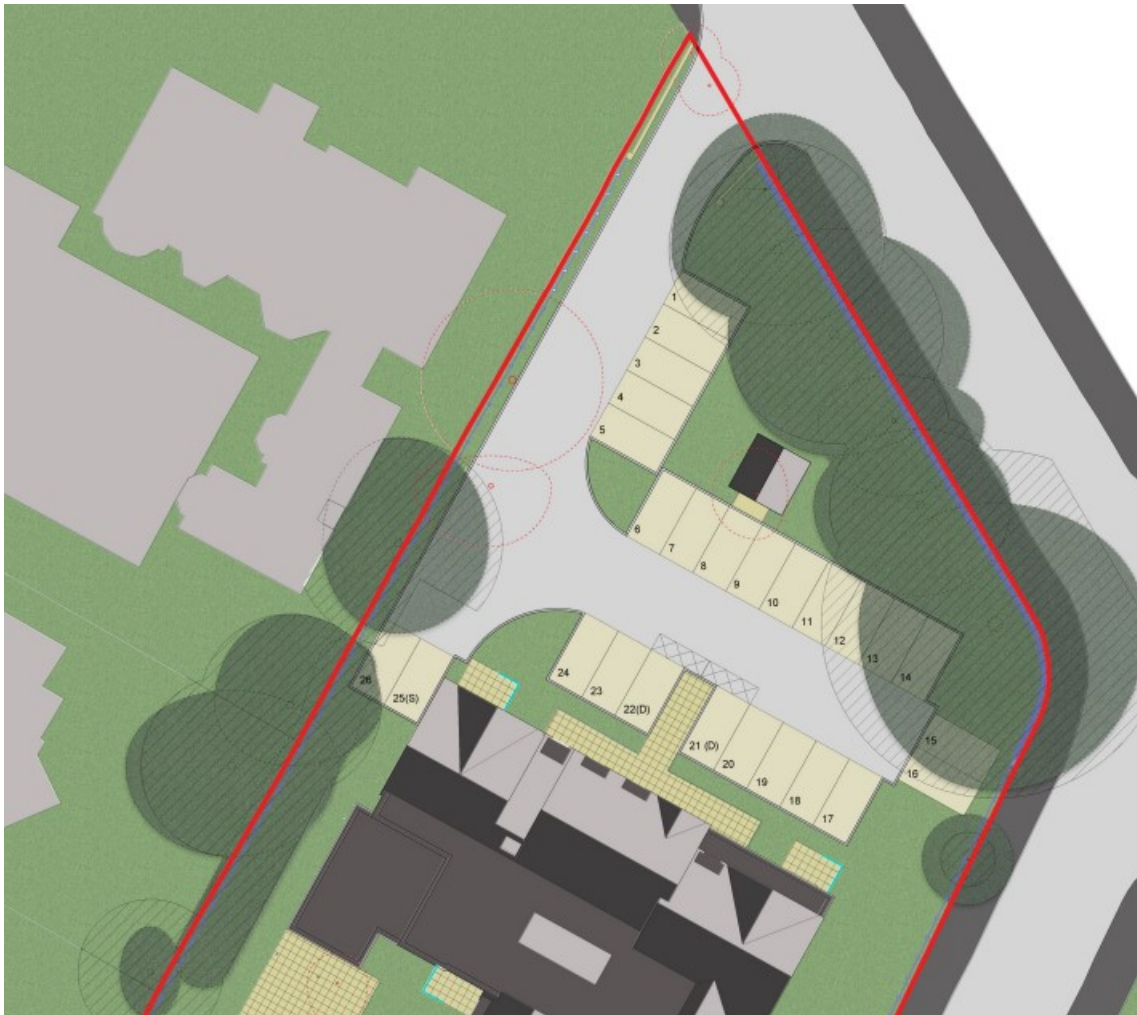
Site plan extract showing a Revised parking layout with 26 spaces, representing 100% provision
